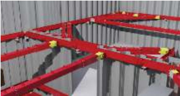
Figure 7. BIM model of temporary framing for excavation [14]
