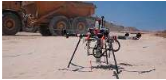
Fig.7: CivDrone Setting Out Product [11]
